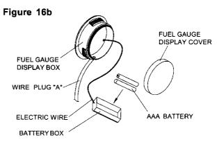
IMPORTANT: When the gas tank is removed from the tank pull-out tray, the fuel gauge display will not operate.
